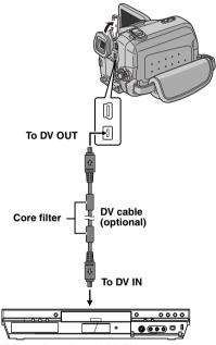
Video unit equipped with DV connector
